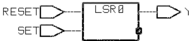
Figure 14-1 Synthesized Design for an SR Latch
